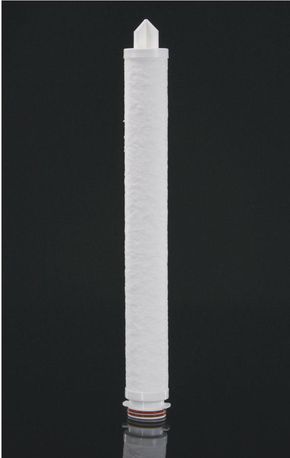
Graded density, high porosity, SPUNFLOW QN filter elements are manufactured from thermally bonded Polypropylene microfibers. Offering high throughputs, low pressure loss, high dirt capacity and long onstream life, the bonded fibre construction minimizes any possibility of fibre migration and is rugged enough to resist particle shedding, even under pulse conditions.
